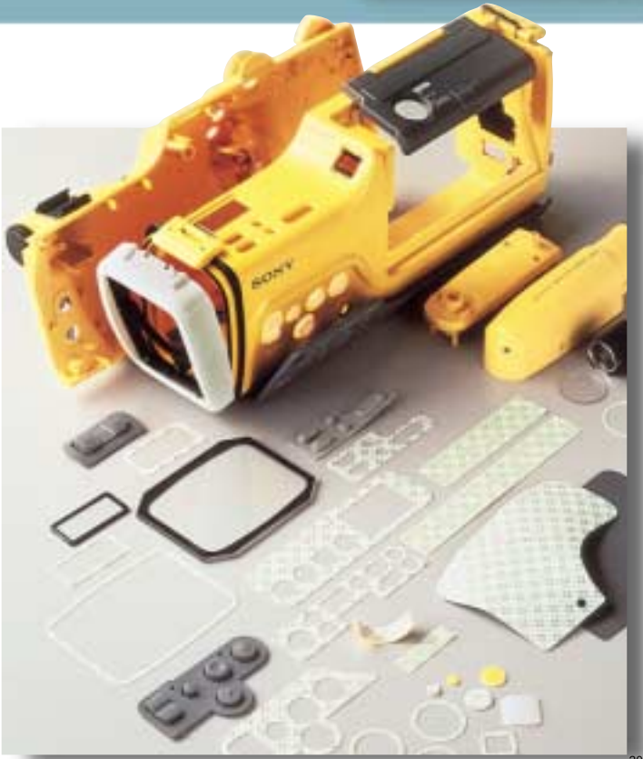
For assembly efficiency, die-cut pieces of 3M™ VHB™ Tape bond components in a water-resistant video camera case. The foam conforms to help seal the unit.
