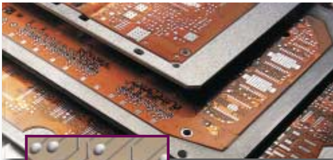
Bond rigidizer to flex circuit and withstand process heat.
