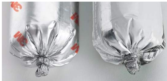
Crimped ends on 3M sausage packs (versus wire clips on other brands) help extend shelf life by sealing out moisture, which can cause premature curing and wasted product
